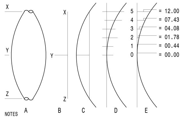
A THE BARREL TO BE TURNED SHOWING THE MAXIMUM AND MINIMUM DIAMETERS B MAXIMUM (Y) AND MINIMUM (X & Z) DIAMETER POSITIONS MARKED C CIRCLE DRAWN BASED ON THE THREE POSITIONS (X, Y & Z) D THE FIVE TOOL INFEED POSITIONS MARKED E LINES TRIMMED AND THEIR LENGTHS (TOOL INFEED)REQUESTED
