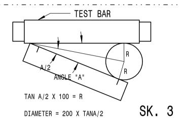
CALCULATION OF DIAMETER FOR ANGLE "A"
