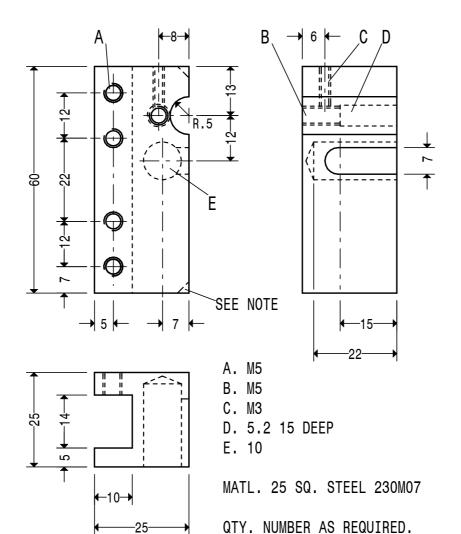
NOTE. IF THE BODY IS BEING MADE TO ACCEPT TWO HOLDERS TWO CORNERS WILL NEED A 3MM CHAMFER, AS SHOWN DOTTED.
