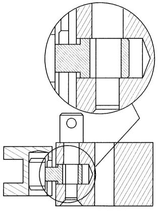
NOTE HOW, IN THE CLAMPED POSITION, THE HOLE IN THE OPERATING PIECE (31) DOES NOT ALIGN WITH THAT IN THE BODY (1). THIS MUST BE TAKEN ACCOUNT OF WHEN USING THE BODY AS A DRILLING JIG FOR DRILLING THE OPERATING PIECE.
